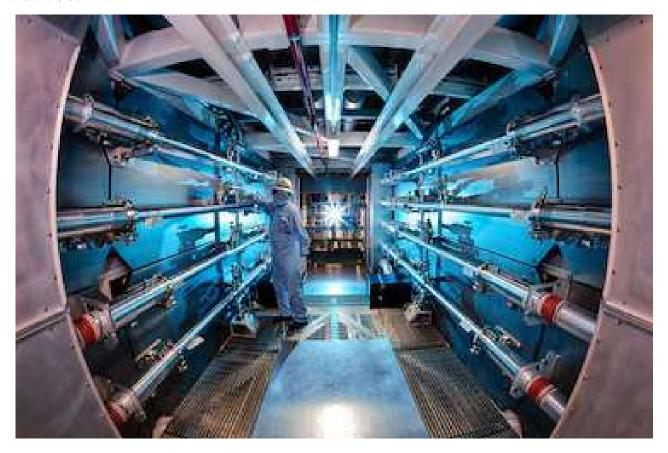
The fusion record was achieved at the National Ignition Facility at California's Lawrence Livermore National Laboratory, which ignites fusion fuel with an array of 192 lasers. These lasers reach high energies thanks in part to devices called preamplifiers (seen here).
